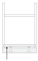
The 1/2" opening between the toe kick and bottom panel facilitates optimal airflow and ventilation efficiency.
